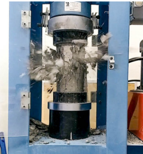
Rupture of cylindrical specimen in a hydraulic press
