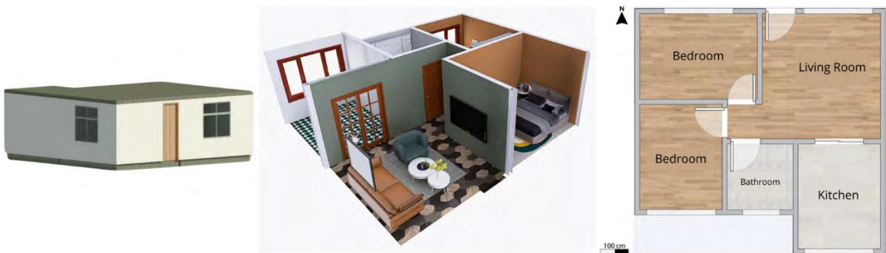
Figure 7 – Simulated residence. Left: external 3D model. Middle: internal 3D model. Right: floor plan.
